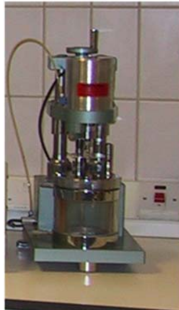
Figure 1 Jack Deer's Air Turbine Rheometer (left); Deer Rheometer (right).
