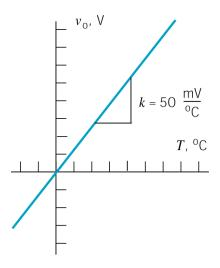
A voltage  $v_0 = 1.5 \text{ V} = 1500 \text{ mV}$  indicates a temperature  $T = \frac{1500}{50} = 30 \text{ °C}$ .
