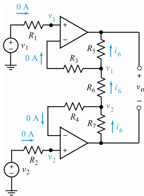
**P2** Use the properties of the ideal op amp to label the circuit as shown.
