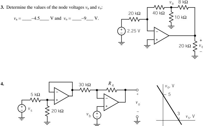
The input to this circuit is the voltage,  $v_s$ . The output is the voltage  $v_o$ . The voltage  $v_b$  is used to adjust the relationship between the input and output. Determine values of  $R_4$  and  $v_b$  that cause the circuit input and output have the relationship specified by the graph
