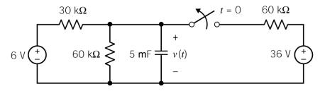
The capacitor voltage is  $v(t) = A - Be^{-at}$  for  $t \ge 0$ . Determine the values of the constants A, B, and a:
