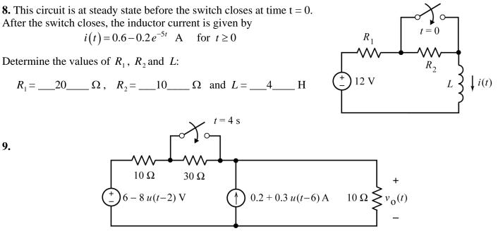
Determine  $v_0(1)$ ,  $v_0(3)$ ,  $v_0(5)$ , and  $v_0(7)$ ; the values of the voltage  $v_0(t)$  at times t = 1, 3, 5 and 7 seconds.
