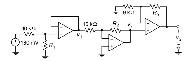
The values of the node voltages  $v_1$ ,  $v_2$  and  $v_0$ , are  $v_1 = 80$  mV,  $v_2 = -320$  mV and  $v_0 = -960$  mV. Determine the value of the resistances  $R_1$ ,  $R_2$  and  $R_3$ :
