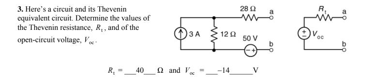
**4.** Here's a circuit and its Thevenin equivalent circuit. Determine the values of the Thevenin resistance,  $R_t$ , and of the open-circuit voltage,  $V_{oc}$ .
