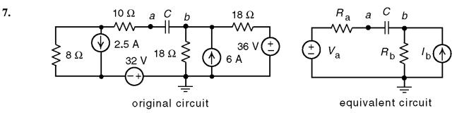
The equivalent circuit on the right is obtained from the original circuit on the left using source transformations and equivalent resistances. (The lower case letters *a* and *b* identify the nodes of the capacitor in both the original and equivalent circuits.) Determine the values of  $R_a$ ,  $V_a$ ,  $R_b$  and  $I_b$  in the equivalent circuit:
