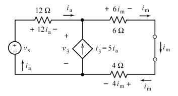
Apply KCL at the top node of the dependent source to write
