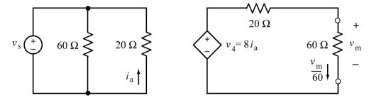
Label the voltages across parallel elements and the currents in series elements.
