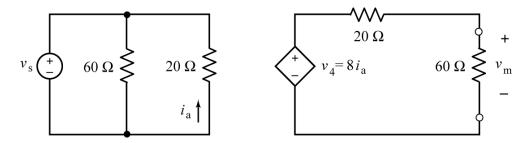
Use Ohm's law to label the current in the 60  $\Omega$  resistor on the right side of the circuit.
