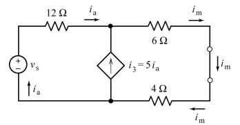
Label the resistor voltages using Ohm's law.
