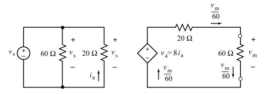
Use Ohm's law to label remaining resistor currents and voltages.
