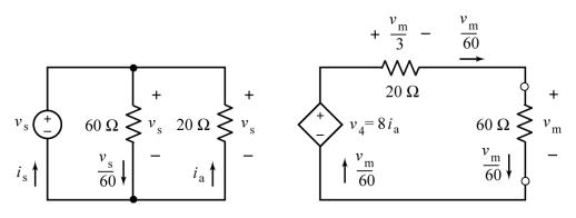
Notice that  $i_a$  and  $v_s$ , the current and voltage of the vertical 20  $\Omega$  resistor, do not adhere to the passive convention. Consequently, Ohm's law gives
