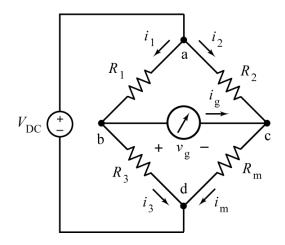
The galvanometer is used to detect the condition  $i_g = 0$ . When the circuit satisfies the condition  $i_g = 0$  we say that "the bridge is balanced".
