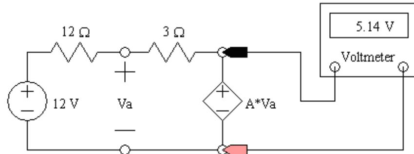
What is the gain of the VCVS, A, in V/V, ?
