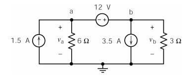
Determine the values of the node voltages,  $v_a$  and  $v_b$ , for this circuit.
