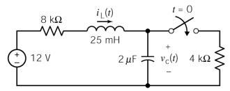
The switch in this circuit has been open for a long time before closing at time t = 0. Find  $v_c(0^+)$ and  $i_{\rm L}(0^+)$ , the values of the capacitor voltage and inductor current immediately after the switch closes. Let  $v_c(\infty)$  and  $i_L(\infty)$  denote the values of the capacitor voltage and inductor current after the switch has been closed for a long time. Find  $v_c(\infty)$  and  $i_L(\infty)$ .
