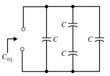
This circuit consists of four capacitors having equal capacitance, C.
