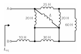
This circuit is equivalent to a single inductor having inductance  $L_{eq} = 18$  H. Determine the value of the inductance L.
