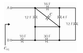
This circuit is equivalent to a single capacitor having capacitance  $C_{eq} = 8$  F. Determine the value of the capacitance C
