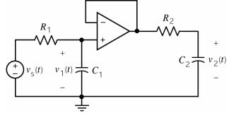
Derive the second order differential equation that shows how the output of this circuit is related to the input.
