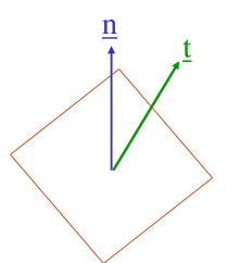
The symbol <u>n</u> represents the unit normal (vector) to the area element, and <u>t</u> is the stress vector acting on that element. The second-order tensor  $\underline{T}$  completely describes the state of stress at a point. By convention, <u>t</u> is the stress exerted **by** the fluid into which <u>n</u> points **on** the fluid adjoining it.
