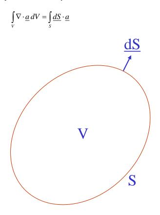
The vector field  $\underline{a}$  should be continuous and differentiable. The symbol  $\underline{dS}$  represents a vector surface element. If  $\underline{n}$  is the unit normal to the surface,
