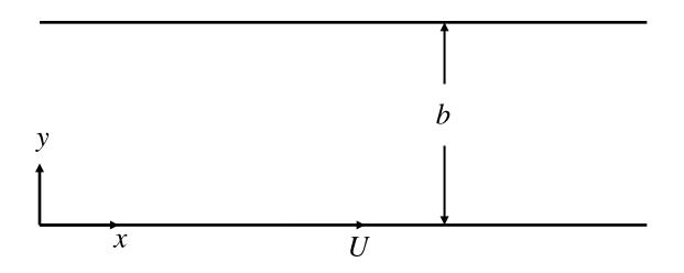
The fluid is initially assumed to be at rest. Motion is initiated by suddenly moving the bottom plate at a constant velocity of magnitude U in the x-direction. The velocity of the bottom plate is maintained at that value for all future values of time t while the top plate is held fixed in place. There is no applied pressure gradient, with motion being caused strictly by the movement of the bottom plate.
