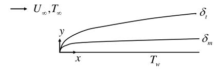
For gases, the Prandtl number is typically of O(1), while for common liquids Prandtl numbers are found to vary from 10 to 1000. The Prandtl numbers of very viscous liquids such as polymer melts can be even larger than 1000, reaching values of  $10^5$  or greater. Because liquid metals are great conductors of thermal energy, Prandtl numbers for liquid metals are typically of  $O(10^{-2})$ .
