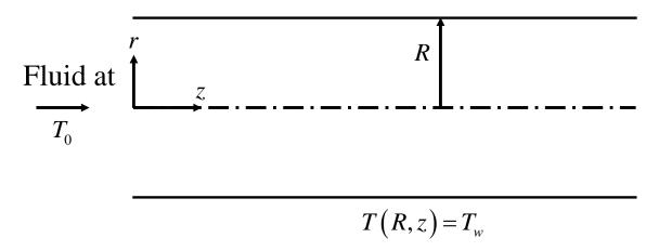
At any given axial position z, the heat flux from the wall to the fluid is given by
