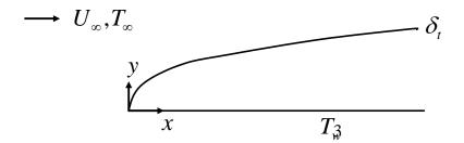
Just as a momentum boundary layer forms at the wall and grows in thickness with distance x along the plate, a thermal boundary layer forms at the wall; the temperature of the fluid changes from  $T_w$  to  $T_\infty$  in the thermal boundary layer. The thickness of the thermal boundary layer  $\delta$ , also grows with distance x.
