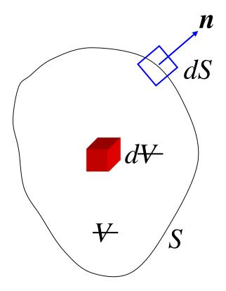
Also marked on the sketch is the bounding surface S of this control volume, called the control surface; an element of surface area dS and the unit outward normal (vector) to that area element, n are shown as well. The vector symbol dS = n dS is used to represent a directed differential area element on the surface.
