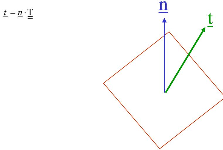
The symbol  $\underline{n}$  represents the unit normal (vector) to the area element, and  $\underline{t}$  is the stress vector acting on that element. The second-order tensor  $\underline{\underline{T}}$  completely describes the state of stress at a point. By convention,  $\underline{t}$  is the stress exerted **by** the fluid into which  $\underline{n}$  points **on** the fluid adjoining it.
