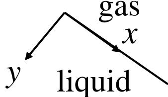
Because the normal velocity is zero at the free surface, the tangential stress balance simplifies to the following result where the subscripts  $l$  and  $g$  represent the liquid and gas, respectively.
