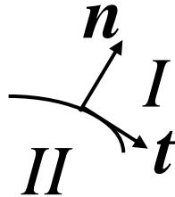
The unit normal vector  $n$  points into phase  $I$  here and the sketch also shows a unit tangent vector to the interface  $t$ .
