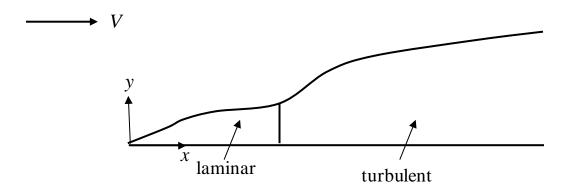
Transition from laminar to turbulent flow in the boundary layer on a flat plate occurs at  $\text{Re}_x \approx 5 \times 10^5$ , where  $\text{Re}_x = xV/v$ . Here, v is the kinematic viscosity of the fluid.
